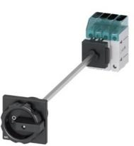
Load disconnector 3LD3, lu 16 A Main switch 3-pole + N Rated operating capacity at AC-23 A at 400V 7.5kW floor mounting Basic switch with door coupling Central hole mounting 22.5mm Rotating drive black 66 x 66 mm
