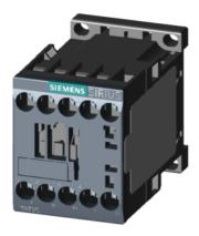
Power contactor, AC-3 9 A, 4 kW / 400 V 2 NO + 2 NC 24 V AC, 50 Hz 4-pole Size S00 screw terminals
