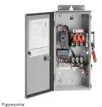
Slim Line Pump Control Panel NEMA size 1 Three phase full voltage Solidstate overload relay OLR amp range 5.5-22A 460VAC 60Hz Coil 30A fusible disconnect 30A/600V fuse clip 1NC / 1NO auxiliary contacts HOA Sel. Sw. <(>&<)> Start/Stop 3-point power terminal block 3-point control terminal block 3-point ground lug Enclosure NEMA type 3/3R Weather proof outdoor use
