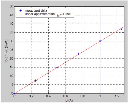
Figure 2 Typical magnetization curve, measured under field oriented control conditions at a speed of 300 RPM
