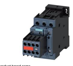
Power contactor, AC-3 38 A, 18.5 kW / 400 V 2 NO + 2 NC, 24 V DC with plugged-in diode combination, 3-pole Size S0, Screw terminal Captive auxiliary switch
