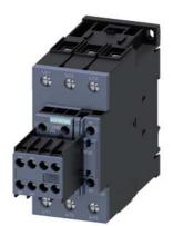
power contactor, AC-3 40 A, 18.5 kW / 400 V 2 NO + 2 NC, 24 V AC 50 Hz, 3-pole, Size S2, screw terminal
