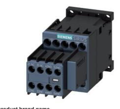
Power contactor, AC-3 9 A, 4 kW / 400 V 3 NO + 2 NC, 110 V AC 50 / 60 Hz, 3-pole, Size S00, screw terminal Varistor plugged on
