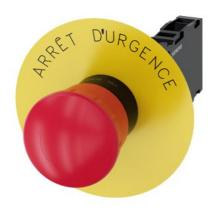
EMERGENCY STOP mushroom pushbutton, 22 mm, round, plastic, red, 40 mm, positive latching, acc. to EN ISO 13850, rotate-to-unlatch, with yellow backing plate, inscription: Arrêt d'urgence, with holder, 1 NO+1 NC, screw terminal, Z=20-unit packaging
