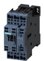
Power contactor, AC-3 25 A, 11 kW / 400 V 2 NO + 2 NC 72 V DC, pole reversing 4-pole size S0 Spring-type terminals 1 NO + 1 NC integrated Traction contactor, integrated varistor
