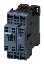
power contactor, AC-3 17 A, 7.5 kW / 400 V 1 NO + 1 NC, 24 V DC with plugged-in diode combination, 3-pole, Size S0 Spring-type terminal
