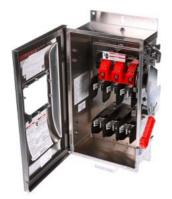
Siemens Low Voltage Circuit Protection Heavy Duty Safety Switches. Type: ENCLOSED, SAFETY SWITCH Std: UL V. Rating: 600V A. Rating: 200A No. Of Poles: 3P F. Rating: 60Hz Action: SINGLE THROW Material: SS Enclosure: TYPE 4X. 2-3 point mounting holes. Insulation: YES O. Cycles: 8000 O. Temperature: (-20F-120F) AMBIENT TEMPERATURE Environmental Conditions: INDUSTRIAL CORROSIVE RESISTANCE
