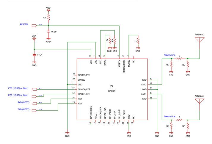
Fig. 2.1. Reference Peripheral Circuit Diagrams
