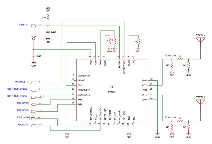
Fig. 2.2. Reference Peripheral Circuit Diagrams
