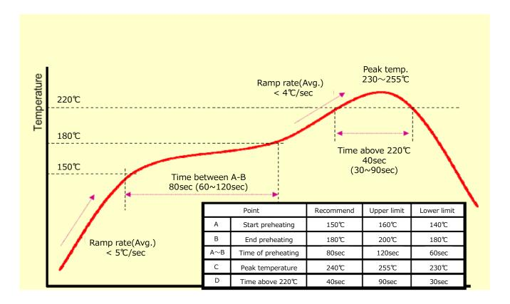
Fig.7. Recommended Reflow Profile
