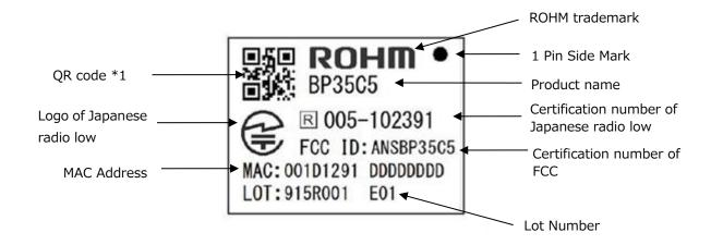
Fig. 4. Marking Specification
