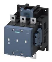
vacuum contactor, AC-3 265 A, 132 kW / 400 V AC (50-60 Hz) / DC operation 200-277 V AC/DC auxiliary contacts 2 NO + 2 NC 3-pole, frame size S10 busbar connections drive: electronic with PLC interface 24 V DC
