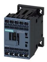
Power contactor, AC-3 16 A, 7.5 kW, 400 V 2 NO + 2 NC 110 V DC 4-pole Size S00 Spring-type terminals
