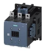
power contactor, AC-3 500 A, 250 kW / 400 V AC (50-60 Hz) / DC 21-27.3 V AC/DC auxiliary contacts 2 NO + 2 NC 3-pole, frame size S12 busbar connections drive: electronic with PLC interface 24 V DC screw terminal
