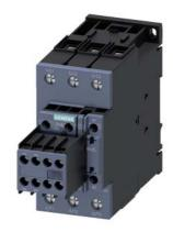
power contactor, AC-3 51 A, 22 kW / 400 V 2 NO + 2 NC, 100 V AC, 50 Hz / 100-110 V, 60 Hz, 3-pole, size S2, screw terminal
