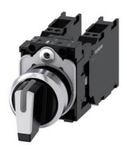
Selector switch, illuminable, 22 mm, round, metal, shiny, white, selector switch, short, 3 switch positions I-O-II, latching, actuating angle  $2x45^{\circ}$ , 10:30h/12h/13:30h, with holder, 2 x 1 NO+1 NC, spring-type terminal, Z=20-unit packaging
