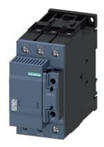
Capacitor contactor, AC-6b 50 kVAr, / 400 V 1 NO + 1 NC, 220 V AC, 50/60 Hz 3-pole, Size S2 screw terminal
