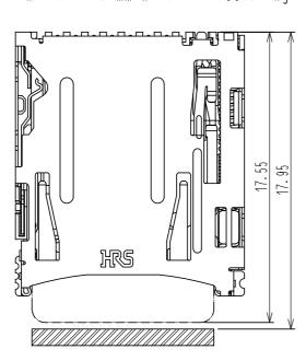
Markings for preventing incorrect card insertion If you will be displaying markings or instructions to prevent end users from inserting the card incorrectly, please pay extra attention to the text description and the direction of the marking used to indicate the correct direction. Recommended finger indent
