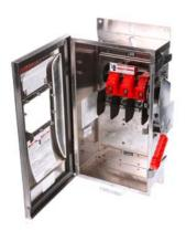
Siemens Low Voltage Circuit Protection Heavy Duty Safety Switches. Type: ENCLOSED, SAFETY SWITCH Std: UL V. Rating: 600V A. Rating: 30 A No. Of Poles: 3P F. Rating: 60Hz Action: SINGLE THROW Material: SS Enclosure: TYPE 4X. 2-3 point mounting holes. Insulation: YES O. Cycles: 10000 O. Temperature: (-20F-120F) AMBIENT TEMPERATURE Environmental Conditions: INDUSTRIAL CORROSIVE RESISTANCE
