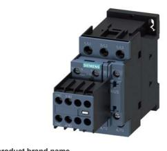
power contactor, AC-3 25 A, 11 kW / 400 V 2 NO + 2 NC, 230 V AC, 50 / 60 Hz, 3-pole, Size S0, screw terminal Removable auxiliary switch
