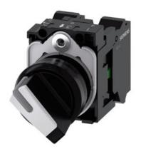
Selector switch, illuminable, 22 mm, round, plastic, white, selector switch, short, 2 switch positions O-I, latching, 10:30h/13:30h, with holder, 1 NO, 1 NC, spring-type terminal, Z=20-unit packaging
