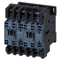
Reversing contactor assembly AC-3,11 kW/400 V,AC24V,50/60 Hz 3-pole, Size S0 Spring-type terminal electrical and mechanical Interlock 2 NO integrated
