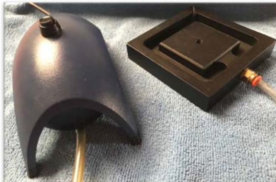
Figure 4. Vacuum pump connected to vacuum fixture
