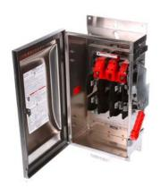
Siemens Low Voltage Circuit Protection Heavy Duty Safety Switches. Type: ENCLOSED, SAFETY SWITCH Std: UL V. Rating: 600V A. Rating: 60A No. Of Poles: 3P F. Rating: 60Hz Action: SINGLE THROW Material: 316SS Enclosure: TYPE 4X. 2-3 point mounting holes. Insulation: YES O. Cycles: 10000 O. Temperature: (-20F-120F) AMBIENT TEMPERATURE Environmental Conditions: INDUSTRIAL CORROSIVE RESISTANCE
