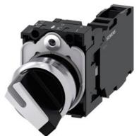
Selector switch, illuminable, 22 mm, round, metal, shiny, white, selector switch, short, 2 switch positions O-I, latching, actuating angle 90°, 10:30h/13:30h, with holder, 1 NO+1 NC, screw terminal, Z=20-unit packaging
