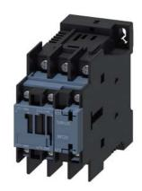
power contactor, AC-3 17 A, 7.5 kW / 400 V 1 NO + 1 NC, 72 V DC with integrated varistor 3-pole, size S0, ring cable lug connection suitable for PLC outputs not expandable with auxiliary switch
