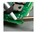
You want to have the pump tip right on top of the joint the best you can with the smallest gap possible for best results. If there just isn't enough room you can remove the iron and put it right over the center as long as you're quick about it.
