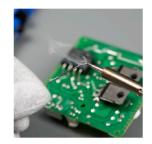
With the solder on your iron tip, pick up the pump and make sure it's loaded and ready.
