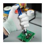
As soon as you see the solder getting molten all around the joint, bring in the pump and place the tip over the joint on the opposite side. The tip is heat-resistant plastic so it shouldn't contaminate the joint or your iron.
