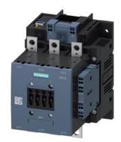
power contactor, AC-3 185 A, 90 kW / 400 V AC (50-60 Hz) / DC operation 96-127 V AC/DC auxiliary contacts 2 NO + 2 NC 3-pole, frame size S6 busbar connections drive: electronic with PLC interface 24 V DC spring-loaded terminal
