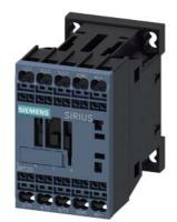
Power contactor, AC-3 9 A, 4 kW / 400 V 1 NC, 125 V DC, 3-pole, Size S00 Spring-type terminal
