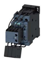
Capacitor contactor, AC-6b 16.7 kVAr, / 400 V 1 NO + 2 NC, 110 V DC 3-pole, Size S0 screw terminal
