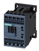
Contactor, AC-3, 7.5 KW / 400 V, 1 NC, 110 V AC, 50 / 60 Hz, 3-pole, Size S00 Spring-type terminal
