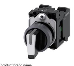
Selector switch, illuminable, 22 mm, round, plastic with metal front ring, white, selector switch, short, 3 switch positions I-O-II, latching, actuating angle 2x45°, 10:30h/12h/13:30h, with holder, 1 NO, 1 NO, spring-type terminal, with laser labeling, upper case and lower case, always upper case at the beginning of the word
