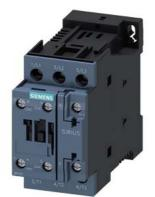
Power contactor, AC-3 32 A, 15 kW / 400 V 1 NO + 1 NC, AC 50-60 Hz / DC 95-130 V AC / DC 3-pole, size S0 screw terminals
