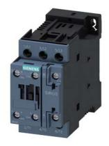
Power contactor, AC-3 38 A, 18.5 kW / 400 V 1 NO + 1 NC, 220 V DC 3-pole, size S0 screw terminals
