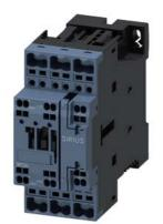
Power contactor, AC-3 32 A, 15 kW / 400 V 1 NO + 1 NC, 24 V DC communication-capable, 3-pole Size S0, Spring-type terminals
