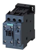
Power contactor, AC-3 32 A, 15 kW / 400 V 1 NO + 1 NC, 24 V DC communication-capable, 3-pole Size S0, screw terminals
