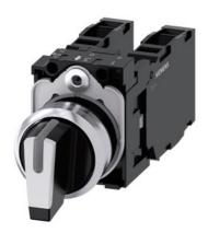
Selector switch, illuminable, 22 mm, round, metal, shiny, white, selector switch, short, 3 switch positions I-O-II, latching, actuating angle  $2x45^{\circ}$ , 10:30h/12h/13:30h, with holder, 2 x 1 NO+1 NC, screw terminal, Z=20-unit packaging
