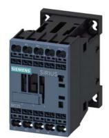
Power contactor, AC-3 12 A, 5.5 kW / 400 V 2 NO + 2 NC 24 V DC 4-pole Size S00 Spring-type terminals
