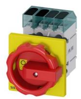
Load disconnector 3LD3, lu 40 A Main switch 3-pole + N Rated operating capacity at AC-23 A at 400 V 18.5 kW Front plate mounting Basic switch with Central hole mounting 22.5mm Toggle drive red / yellow 66x66 mm
