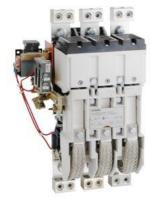
Mechanically held lighting contactor, Contactor amp rating 400A, 0 N.C. / 3 N.O. poles, 277VAC 60HZ coil, Non-combination type, Enclosure NEMA type (open), No enclosure
