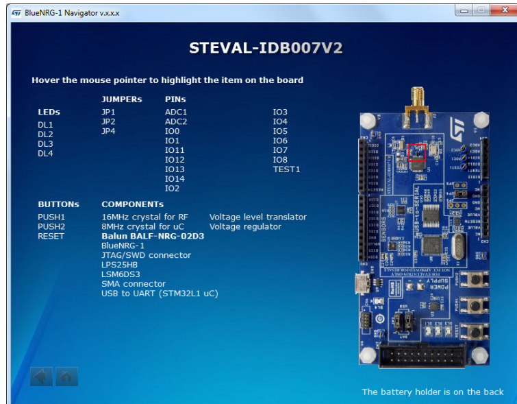
Figure 18. STEVAL-IDB007V2 kit components
