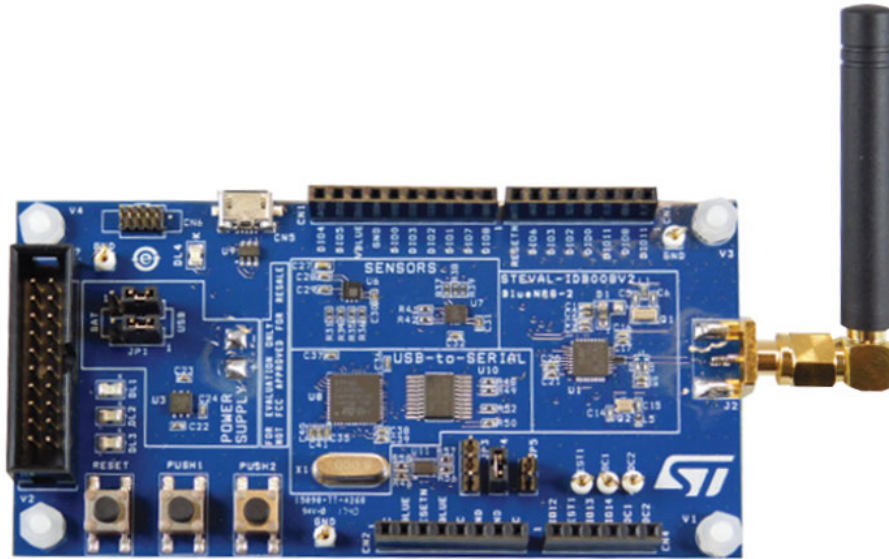
Figure 5. STEVAL-IDB009V1 development platform
