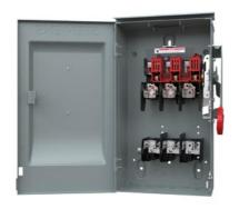
Siemens Low Voltage Circuit Protection Heavy Duty Safety Switches - Type ENCLOSED / SAFETY SWITCH Meets stds: UL. Built material: 304SSsingle throw action. Rated 600VDC (30A) at 60Hz.3-Pole. Insulated. TYPE 3R enclosure with 2 or 3 point mounting. No special features listed.
