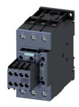
Power contactor, AC-3 65 A, 30 kW / 400 V 2 NO + 2 NC, 48 V AC, 50/60 Hz 3-pole, size S2 screw terminals
