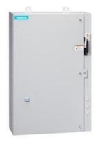
Non-reversing motor starter, Size 2 1/2, Three phase full voltage, Solid-state overload relay, OLR amp range 25-100A, 240V 50Hz / 277V 60Hz coil, Combination type, 60A fusible disconnect, 60A/600V fuse clip, Enclosure NEMA type 4/12, Water/dust tight for outdoors, Extra-wide enclosure
