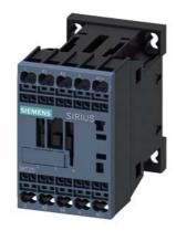
Power contactor, AC-3 12 A, 5.5 kW / 400 V 2 NO + 2 NC 48 V DC 4-pole Size S00 Spring-type terminals integrated diode
