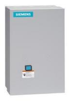
Non-reversing motor starter, Size 2 1/2, Three phase full voltage, Amb. compensate bimetal OLR, Contactor amp rating 60A, 240V 50Hz / 277V 60Hz coil, Non-combination type, Enclosure type 1, Indoor general purpose use
