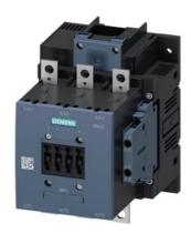
power contactor, AC-3 115 A, 55 kW / 400 V AC (50-60 Hz) / DC operation 575-600 V AC/DC auxiliary contacts 2 NO + 2 NC 3-pole, frame size S6 busbar connections drive: conventional screw terminal
