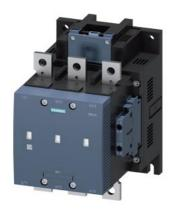
vacuum contactor, AC-3 300 A, 160 kW / 400 V, AC (50-60 Hz) / DC operation 200-277 V AC/DC auxiliary contacts 2 NO + 2 NC 3-pole, frame size S10 busbar connections drive: electronic with SPS interface DV 24 V
