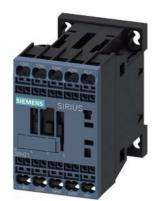
Coupling contactor relay, 3 NO + 1 NC, 30 V DC, 0.7 ... 1.25\* US, with integrated diode, Size S00, Spring-type terminal suitable for PLC outputs
